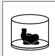
6. Place the impression securely in a duplicating flask/investment form suitable for the chosen manufacturing process
