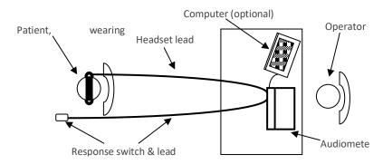
The patient is seated in front of the desk facing away from the operator. The patient wears a headset (see Section 4.3) and responds to test stimuli by use of a hand-held switch which is also connected to the instrument.
